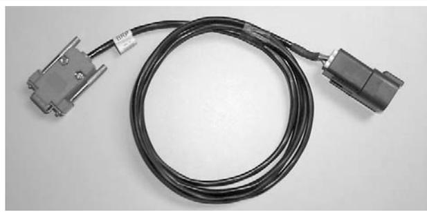
NOTE: AN EXTENSION CABLE AVAILABLE AT ELECTRONIC RETAIL OUTLETS CAN BE USED. DO NOT EXCEED 7.6 M (25 FT).
